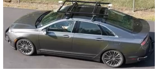
Figure 8: The full-sized sedan used for the RL-MPC on-board testing; equipped with drive-by-wire system, Polynav 2000P GNSS-inertial system, a Calmcar front view camera, and a Dspace Autera computing unit.
